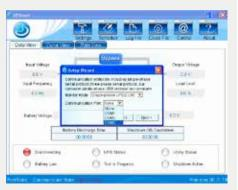
Choose communication port: when choose "single-phase UPS(COM)", If the device and the computer is good at this moment, can be detected in communication port automatically connect a serial port, as shown in figure choose COM3 port, click next after a connection is set.
