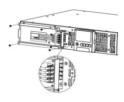
Step 4: Fasten back the connectors on the battery retaining cover. Then insert the battery connectors and tighten the screws of battery retaining cover
