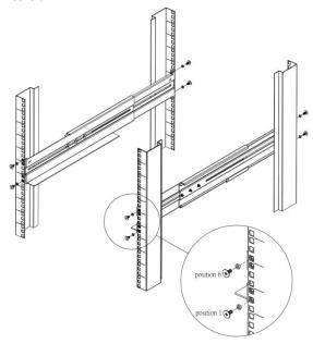
Place the UPS on a flat stable surface with the front of the unit facing toward you. Secure the UPS to your rack with four M5X12L screws at the front of the rack. (Located in position 2 & position 5)
