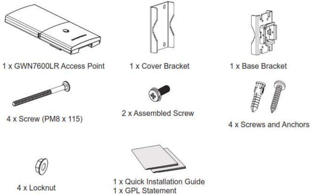
**Figure 1: GWN7600LR Equipment Package**
