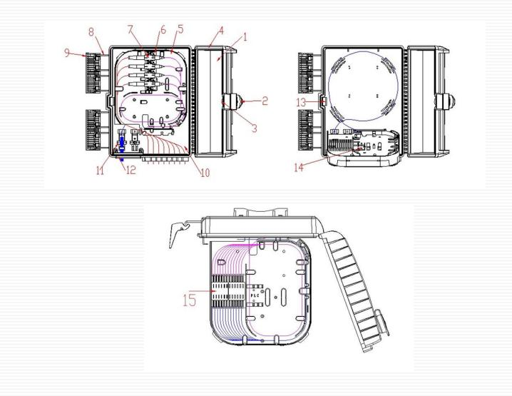
1.Lid; 2.Lock coat; 3.Lock; 4.Seal gasket; 5.Splicing flap plate; 6.Adaptor holder; 7.Adaptor; 8.Lid lock joint bracket; 9.Lid lock clip; 10.Base; 11. Cable strengthen mound layer; 12. Joint (Option); 13.Lock panel; 14.PLC mounting position; 15. Hot tube fixer
