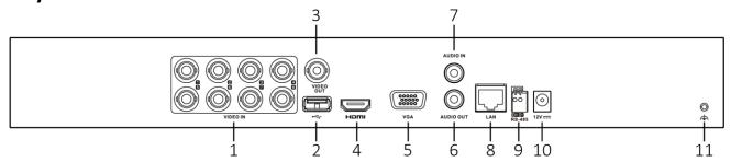
\*: The rear panel of iDS-7204HUHI-M2/S and iDS-7216HUHI-M2/S provide 4 or 16 video input interfaces.
