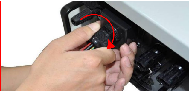
Step 4: Tighten the cable gland in clockwise direction.
