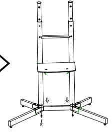
Fix the VESA panel(P1) to the (P2) and (B1) by screw (K) and nut (H).
