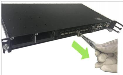
Pulling the optical module (hook end)
