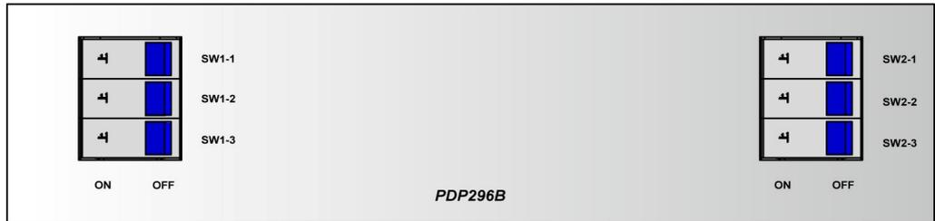
The PDP296B (3000068) has six air automatic circuit breakers on its front panel to control the power supply outputs. Among which:
